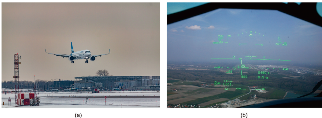
Fig. 2. (a) The radio altimeter is most important when planes are at low altitude, and particularly for landings in low-visibility conditions. (b) The head-up display in an aircraft cockpit projects key flight information such as altitude and air speed onto a screen in the pilot’s line of sight. It is one of the systems that depends on the radio altimeter and could be disrupted by 5G interference. Credits: Vincent Albos (CC0); Joschiki (CC BY-SA 3.0).
